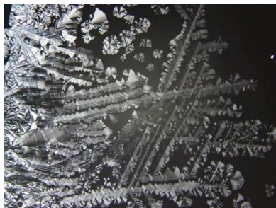
Fig. 2. Lyotropic textures of lecithin with chiral additives, where the rectangular textures are clearly seen.
